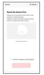
Change 'EZ Mode' to 'AP Mode' by clicking in the top right hand corner Ensure your device's Wifi LED is flashing slowly. If it is not, hold down the timer button for 5 seconds or until the Wifi icon begins to flash. Click 'Confirm indicator slowly blink' and 'Next'
