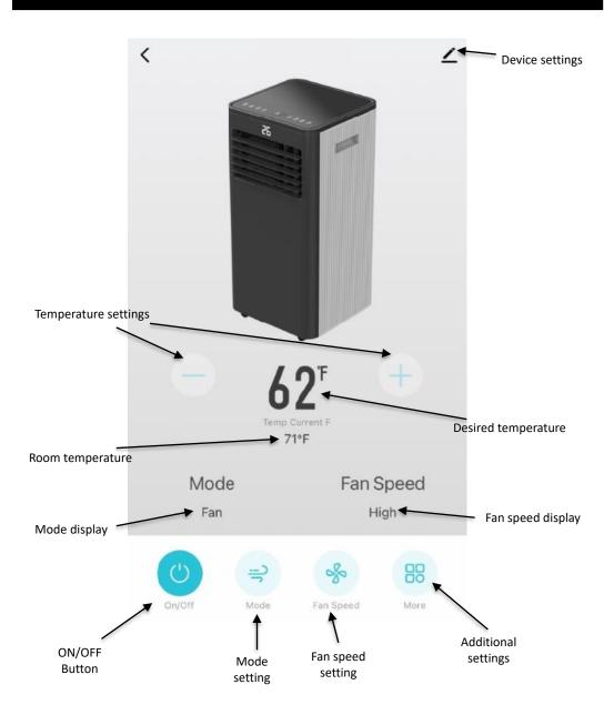
Note: you can change the desired temperature display between Fahrenheit and Celsius in additional settings
